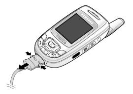
**Note:** You must unplug the charger before removing the battery from the phone during charging, otherwise, the phone could be damaged.
